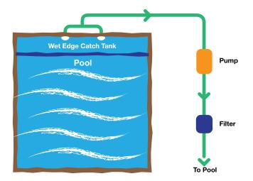
**Problem:** On standard wet-edge pools, there is no skimmer box installed. Therefore there is no easy or safe way to install a suction pool cleaner or to manually vacuum the pool or catch tank.
