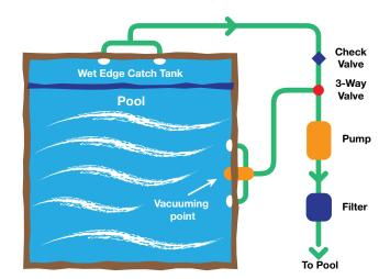
**Solution:** Install the Davbroz Safe-T-Suction. This will provide for a safe vacuum connection point for manual or automatic pool cleaning. A three-way valve and check valve need to be installed.
