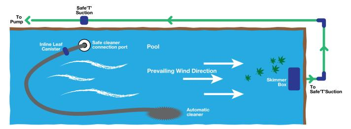
Safe'T'Suction can be installed in conjunction with a skimmer box. Place skimmer correctly to surface skim and locate Safe'T'Suction in the most convenient location to vacuum pool. Speed controlled suction and shorter hose length gives a better result and skimmer can still operate as it was originally designed.
